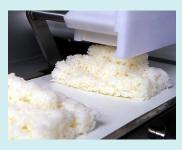
Adding shortage volume of rice for the gap weight by sub-measuring roller unit.
