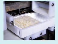
Serving of 80-90% setting weight by measuring roller unit and measuring actual weight by weight checker.
